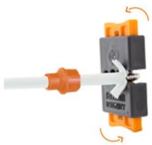
4 Insert the cable in the round hole until the dielectric just peaks on the other side. Rotate the tool + -90° while squeezing the blades to cut and remove the dielectric.
