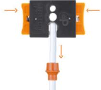
2 Insert the coaxial cable into the side slot of the stripping tool (SPC) about 1cm (3/8"); gently squeeze the blades while pulling the cable out to slit both sides of the jacket.
